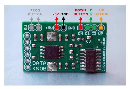
You will need to source +5v and GND to power the board. If you have a mkl synth then here are two options here. The easiest way of doing it is to unscrew the chorus board to the right and wire the power connections to the positions shown at the top of the next page.
