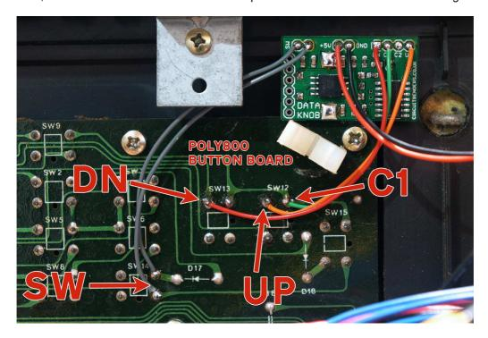
The green common (COM) wire should be soldered to the top right pin of SW12. You can use either the C1 or C2 solder points on the Data Knob PCB for this.
