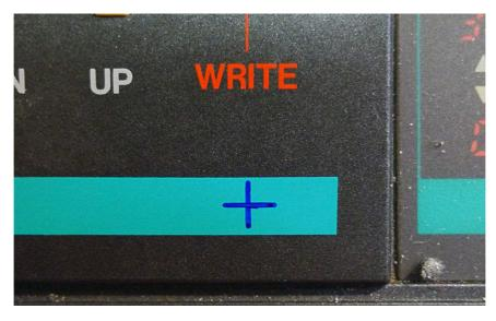
Drill the hole here to mount the knob in the recommended position. Line it up with the red line above 'WRITE', and exactly halfway across the blue bar. This should be as accurate as possible.
